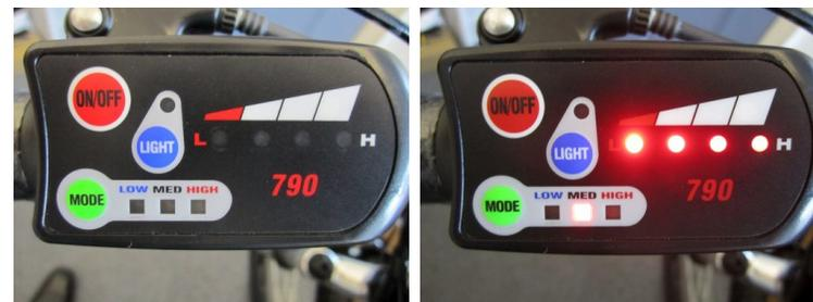
The “On/Off” button turns on the control module, the “Mode” button is used to vary the level of assistance, and the “Light” button is used to turn the lights on/off.
