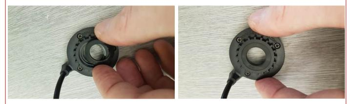
Ensure that your bottom bracket matches the one shown below, and then slide the sensor into position.
