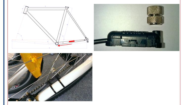
Run the cable along the chain stay as indicated in RED above, securing it with cable-ties and ensuring that the cable is clear of the wheel/tyre. See the next page for the various connections to the controller.
