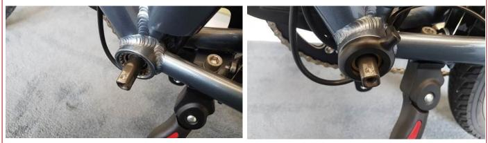
Fit the plastic ring that incorporates the magnets. The silver magnets should face inwards.
