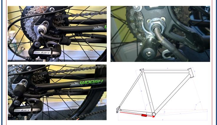
The red arrow on the diagram above shows the usual route for the motor cable, with the quick-release connector (in the cable) indicated by the solid red box.
