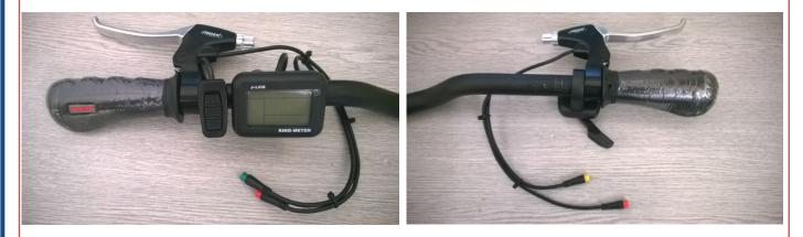
Depending on the configuration of the bike, it may be more practical to mount the throttle and display in slightly different locations or on opposite sides. The next step is to run the modular cable (for the LCD, throttle and brake cut-outs) from the front of the bike back to the controller.
