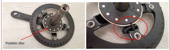
With the sensor in place as per the photo above, it now needs to be secured, the way you achieve this may vary depending on your specific bike. In this example, we're just using some cable-ties.
