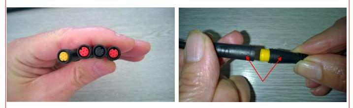
Ensure that the arrows line up on both sides before pushing the connectors firmly together, be careful with them and don't force them or you may bend/damage the pins. Also be sure to mate the cables with the matching coloured connectors.
