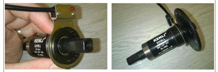
You need to ensure that the disc is the correct way around on the spindle, otherwise you will find that the motor kicks in when you pedal backwards! The disc should be fitted such that the arrows on the disc are on the left side.
