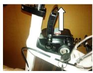
To flip the saddle, simply press the release lever upwards at the rear underside of the saddle and rotate the saddle forwards. This will allow enough clearance to remove the battery.
