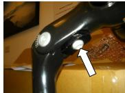
You can now rotate the handlebars upwards/towards the rider. Make sure that the various cables aren't pulled too tightly as this may restrict the turning of the handlebars and/ or damage the cables. When you have adjusted the handlebars to the desired position, tighten the locking piece and then retighten the allen bolts to secure the handlebars in place.
