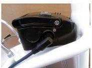
Do not connect the charger to the bike when the charger is already switched on.
