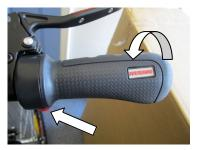
On the left side of the handlebars is the control module. This is used to turn the motor on/off and also to increase/ decrease the amount of assistance given from the electric motor. This module also indicates the **voltage** status of the battery and is used to switch the bike lights on/off.
