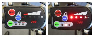
The "On/Off" button turns on/off the control module, the "Mode" button is used to vary the level of assistance and the "Light" button is used to turn the lights on/off.
