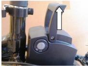
If your bike has the flip-saddle, simply press the release lever on the underside of the saddle and rotate the saddle forwards. This will allow enough clearance to remove the battery. For the standard saddle type, simply undo the clamp and lift the saddle to gain the clearance needed.
