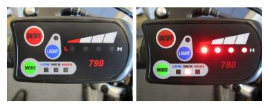
The "On/Off" button turns on/off the control module, the "Mode" button is used to vary the level of assistance and the "Light" button is used to turn the front light on/off.
