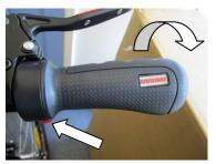
On the left side of the handlebars is the control module. This is used to turn the motor on/off and also to increase/ decrease the amount of assistance given from the electric motor. This module also indicates the **voltage** status of the battery and is used to switch the front bike light on/off.
