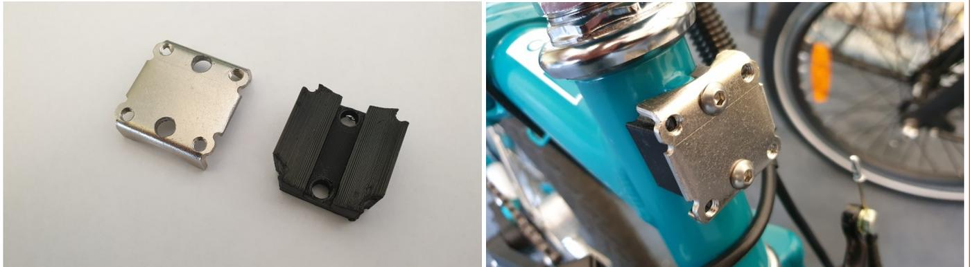
The parts to be fitted next are shown below-left. Drop the white into the rear of the black casing, and feed the four M5 cross-head bolts through the metal support from the other side, and then secure it to the bike. The round opening in the side of the black plastic should be on the left as you look at the bike (the right side if you were sitting on the bike).
