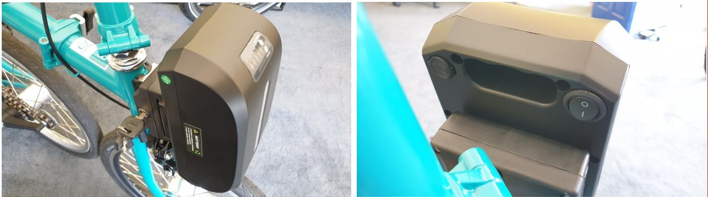
The battery has a meter showing the remaining capacity, and a light which would normally be used when the battery is fitted to the rear of a bike. To see the state of the battery, press the 'Voltage' button, and to switch the light on/off, press the light button. The light will cycle from Off > On > Flashing > Off.
