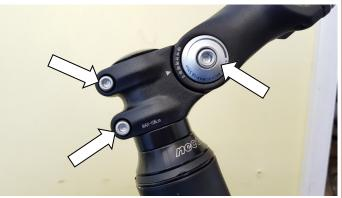
Undo the four bolts and remove the clamp, place the handlebars centrally within the clamp, ensure that none of the cables are twisted, then fit the clamp back in place to secure the bars in position. Also tighten the bolt used for the angle adjustment (see above-right) You can fine-tune the position of the handlebars once the rest of the assembly is complete, but for now, they are out of the way and won't scratch the frame while the bike is prepped.
