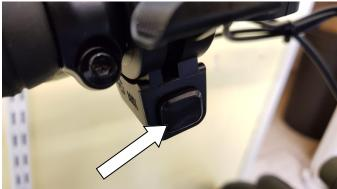
The thumb-throttle cannot be used to start the bike from a standstill, you have to have pedalled first for the throttle to become active. The bike does however feature "start-assist" which is activated by holding the minus (-) button on the display.
