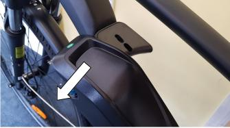
To get a rough idea of the remaining charge in the battery, press the button located at the lower-right side of the battery, the more segments that illuminate, the more remaining capacity there is. All segments illuminated would indicate a full or near full battery.
