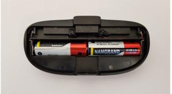
The front lamp uses 2x AA batteries. The on/off button is located on the top face of the lamp. To change the batteries, press down on the small clip at the base of the lamp, and lift the lens/reflector clear. The batteries should be oriented as shown below-right.
