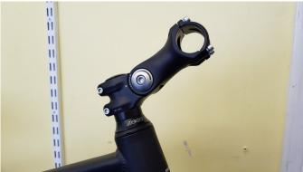
Once the stem is facing the correct way, remove the rubber cover and tighten the stem-bolt with a 5mm Allen key, and then tighten the two bolts (indicated below-right) with a 4mm Allen key, and then proceed with fitting the bar into the clamp.
