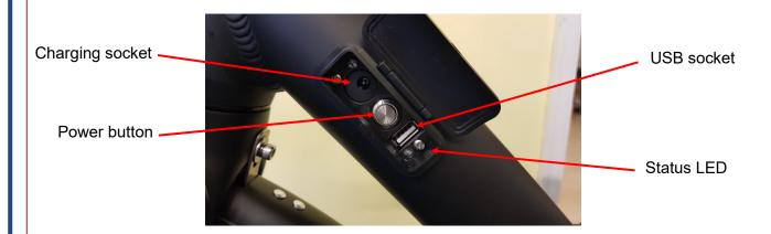
The status LED indicates the current state of the battery. If the LED is not illuminated, the battery is switched off, press the power button switch the battery on. The LED will glow blue when the battery is on. When the battery is powered down, the LED will cycle through red and green for a second or so as the battery switches off—this is normal.
