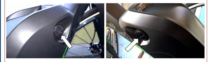
The battery lock is located on the opposite side to the charger socket (see photo above-right) and needs to be turned fully anti-clockwise to unlock the battery. When unlocked, the battery is simply slid upwards towards the front of the bike a little and then it can be lifted clear of the bike. Reverse the procedure to put the battery back on the bike, **do not forget to lock the battery**.
