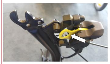
The front wheel features a quick release (QR) system so the wheel can be quickly and easily removed/ refitted.
