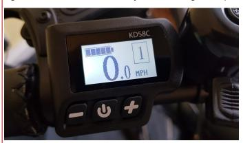
To adjust the assistance level, use the (+) to increase the assistance and (-) to reduce the assistance. There are 5 levels of assistance (1 to 5)
