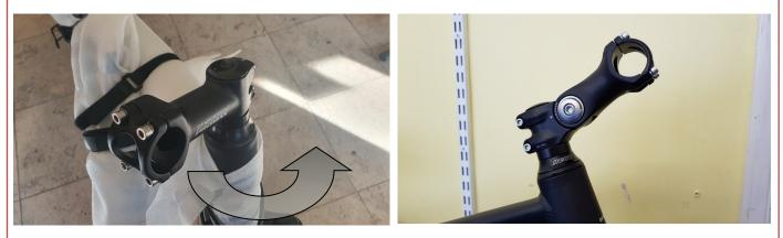
Once the stem is facing the correct way, remove the rubber cover and tighten the stem-bolt with a 5mm Allen key, and then tighten the two bolts (indicated below-right) with a 4mm Allen key, and then proceed with fitting the bar into the clamp.
