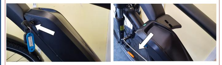
To get a rough idea of the remaining charge in the battery, press the button located at the lower-right side of the battery, the more segments that illuminate, the more remaining capacity there is. All segments illuminated would indicate a full or near full battery.
