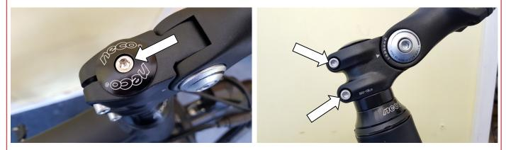
Undo the four bolts and remove the clamp, place the handlebars centrally within the clamp, ensure that none of the cables are twisted, then fit the clamp back in place to secure the bars in position. You can fine -tune the position of the handlebars once the rest of the assembly is complete, but for now, they are out of the way and won't scratch the frame while the bike is prepped.
