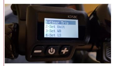
Option 1 - is used to reset the trip back to zero.
