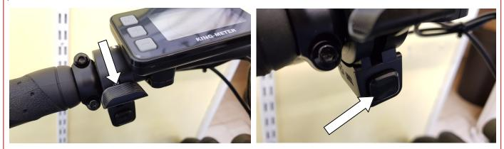
The thumb-throttle cannot be used to start the bike from a standstill, you have to have pedalled first for the throttle to become active. The bike does however feature "start-assist" which is activated by holding the minus (-) button on the display.
