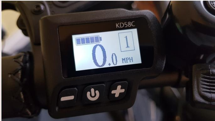
To adjust the assistance level, use the (+) to increase the assistance and (-) to reduce the assistance. There are 5 levels of assistance (1 to 5)
