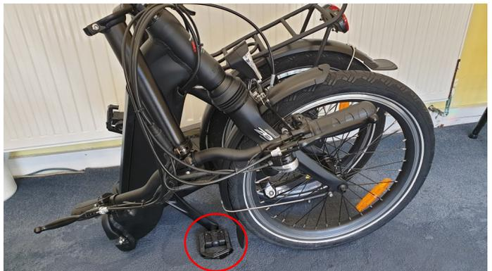
With the clamp disengaged, the bike can be folded. This can be quite cumbersome the first few times, but the more you do it, the easier it becomes. You may need to adjust the position of the cranks so that the pedals don't interfere when you fold the bike. If you leave the left pedal unfolded and the crank in roughly the 4 o'clock position (as shown above-right), it will help with stability when the bike is folded. Alternatively, lean the bike against a solid surface.
