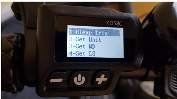
To enter the advanced settings, **press and hold** both the plus and minus buttons for a second or so
