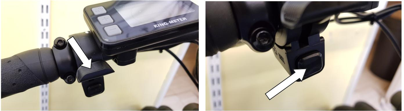
The button underneath is used to enable/disable the twist-grip, the button has two positions, 'in' to enable it, 'out' to disable it.
