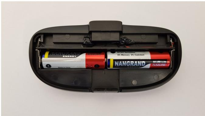
The front lamp uses 2x AA batteries. The on/off button is located on the top face of the lamp. To change the batteries, press down on the small clip at the base of the lamp, and lift the lens/reflector clear. The batteries should be oriented as shown below-right.
