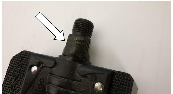
Finger tighten the pedals as much as you can, then tighten the rest of the way using a 15mm spanner.
