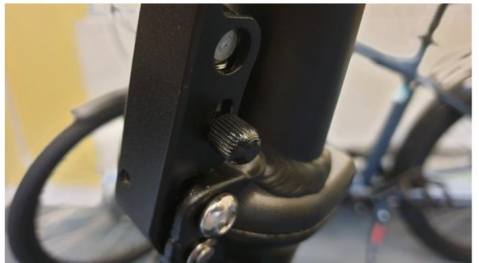
To fold the handlebars, lift the small lever shown above-right to release the clamp mechanism, and pull the clamp downwards and away from the stem.
