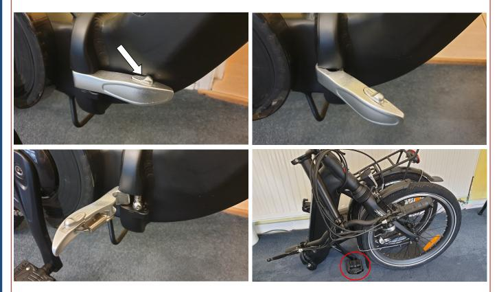
With the clamp disengaged, the bike can be folded. This can be quite cumbersome the first few times, but the more you do it, the easier it becomes. You may need to adjust the position of the cranks so that the pedals don't interfere when you fold the bike. If you leave the left pedal unfolded and the crank in roughly the 4 o'clock position (as shown above-right), it will help with stability when the bike is folded. Alternatively, lean the bike against a solid surface.
