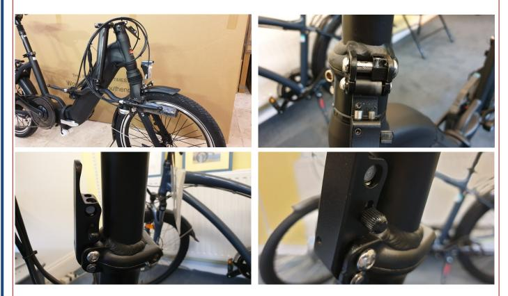
To fold the handlebars, lift the small lever shown above-right to release the clamp mechanism, and pull the clamp downwards and away from the stem.
