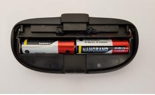
The front lamp uses 2x AA batteries. The on/off button is located on the top face of the lamp. To change the batteries, press down on the small clip at the base of the lamp, and lift the lens/reflector clear. The batteries should be oriented as shown below-right.
