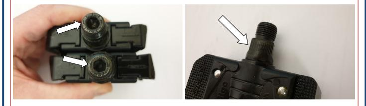
Finger tighten the pedals as much as you can, then tighten the rest of the way using a 15mm spanner.
