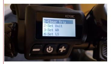
To enter the advanced settings, **press and hold** both the plus and minus buttons for a second or so
