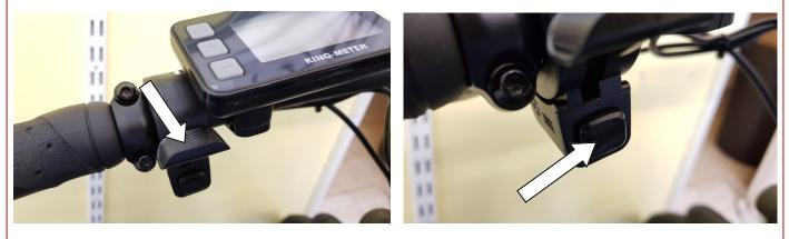
The button underneath is used to enable/disable the twist-grip, the button has two positions, 'in' to enable it, 'out' to disable it.
