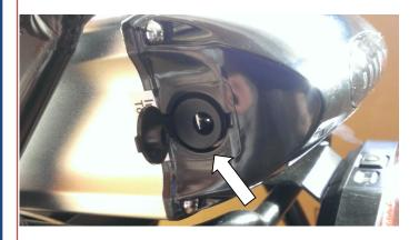
To charge the battery, simply lift the weatherproof cover and connect the charger to the socket and then plug the other end into a regular mains socket. On the charger is a small light which is red while charging. When charging is complete, this light will turn green.
