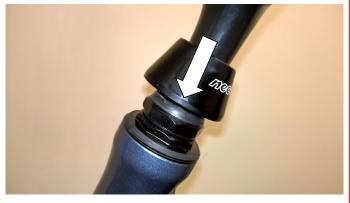
You may have a cap covering the hole where the Allen bolt is, if this is the case, just pull it out, and then put it back once you have fully tightened and adjusted the handlebars.
