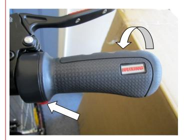
You should ideally ensure that the twist-grip is disabled when mounting/dismounting the bike (or make sure the display is switched off), this is to avoid the situation where you might twist the throttle a little unintentionally and have the bike lurch forward unexpectedly as a result.
